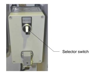
Switch on the unit (switch position "MAN" on the selector switch) and check whether the filter housings are filled with water.
