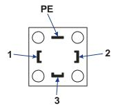
In normal condition: contact 1 and 2 open, contact 1 and 3 closed In alarm condition: contact 1 und 2 closed, contact 1 and 3 open Without main voltage: contact 1 and 2 closed, contact 1 and 3 open
