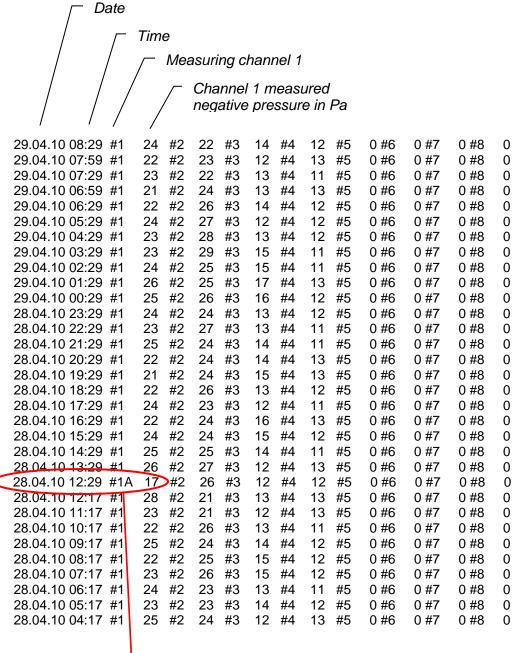
Alarm, marked by "A" behind the measuring channel
