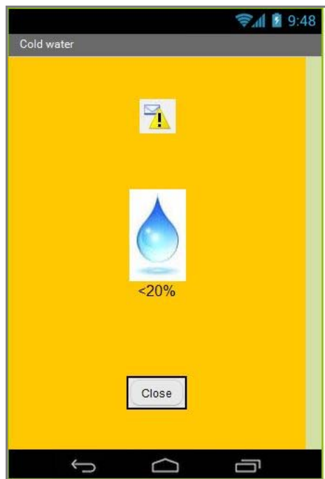
Fig. 1 110 Warning message Filling level of cold water tank below 20%
