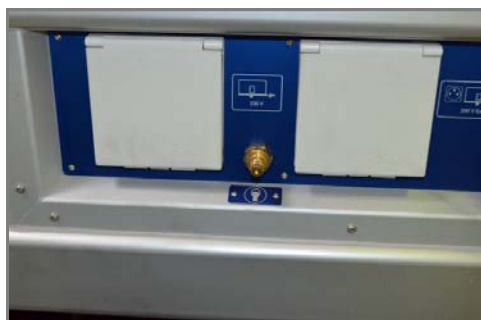
Fig. 1 124 Compressed air feed
