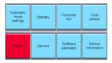
To make the settings and switch automatic mode on/off, tap the "Menu" button. In the following menu, tap the "Automatic mode settings" button.
