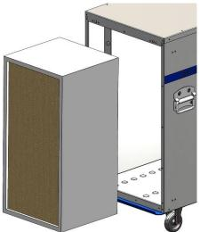
Check and clean the sealing surface on the appliance
