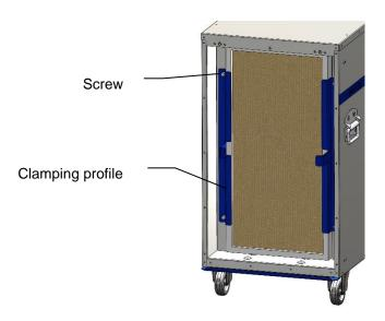
Remove clamping profiles
