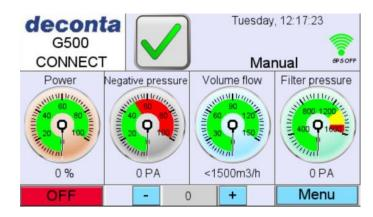
To switch off the device, tap the red "OFF" button
