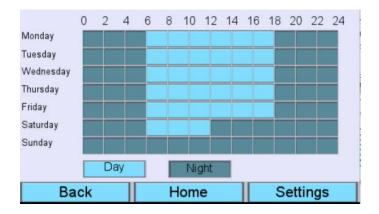
By selecting time ranges, you can set here on which days and at what time the value set in automatic mode for the minimum negative pressure in night mode (min. negative pressure night) is activated.
