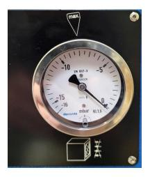
The following table shows the display values for a recommended filter change. If the display reaches this value, please replace the pre-filter first. If the display value drops by 100 Pascal or more, the appliance can continue to be operated. If the value drops by less than 100 Pascal, the HEPA filter must be replaced.
